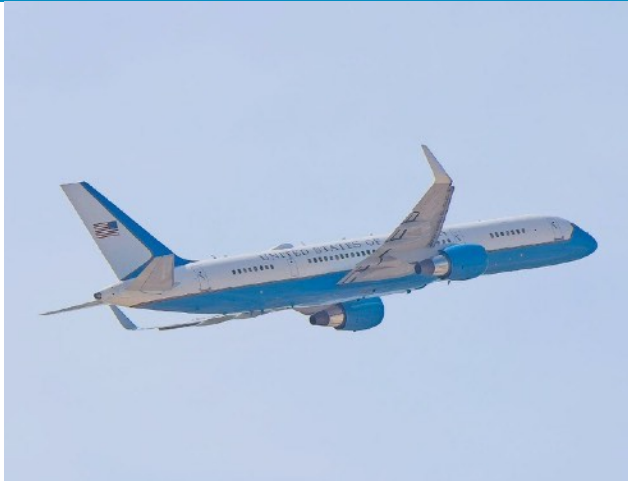
Here is a C32 (USAF B757 VIP transport) taking off out of Abu Dhabi
