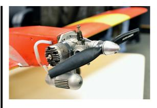
This RC racer has a one-cylinder engine that holds about a thimble full of fuel.
