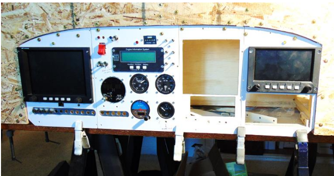
Final panel layout with most components installed. Square hole is for existing radio stack, lower right will be new, more compact glove box. New GRT Sport SX on left will be slaved to older GRT Horizon HZ and become the new primary display.
