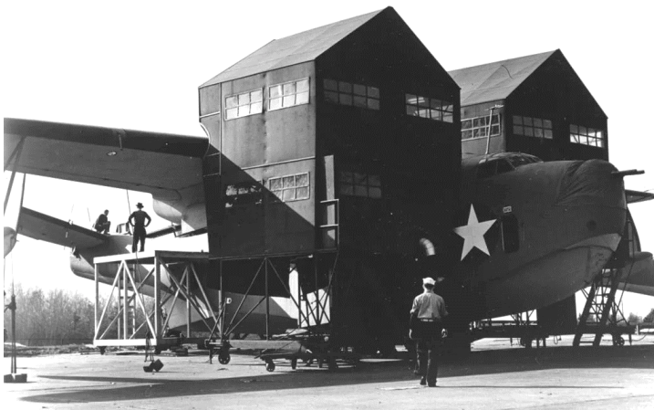
Martin PBM-3D Mariner engine maintenance in cold weather
