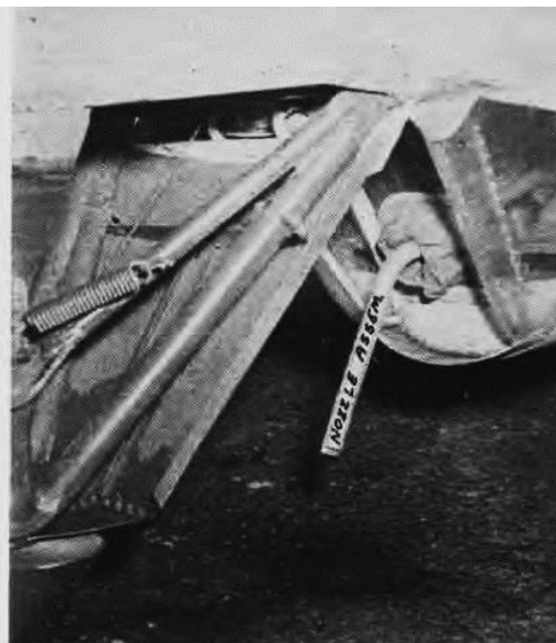
Lethal nozzle replacing tunnel gun in TBM leaves 300 foot swath. Avenger covers 550 acres in one hop at 165 mph ground speed
