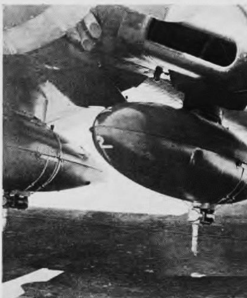
DDT tanks for F4U can be mounted in half hour. Adaptable to several Navy and Army planes, they can be jettisoned for combat
