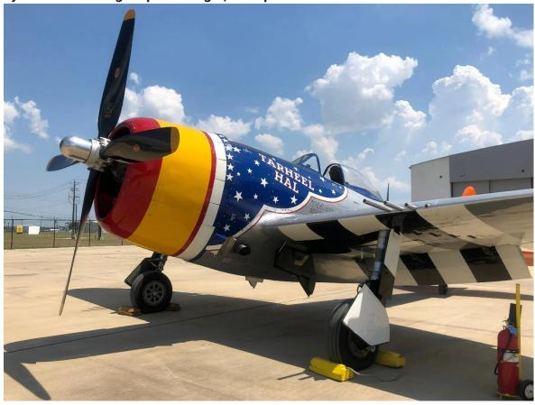
The top speed was 553 MPH with a rage of 800 miles wingspan was 41 feet and they weighed 10,000 #'s First flight was May 6<sup>th</sup> 1941 This was a very competitive aircraft great in air combat and devastating in ground support. With her 8 fifty cal. Machine guns you could add 6 more rockets!
