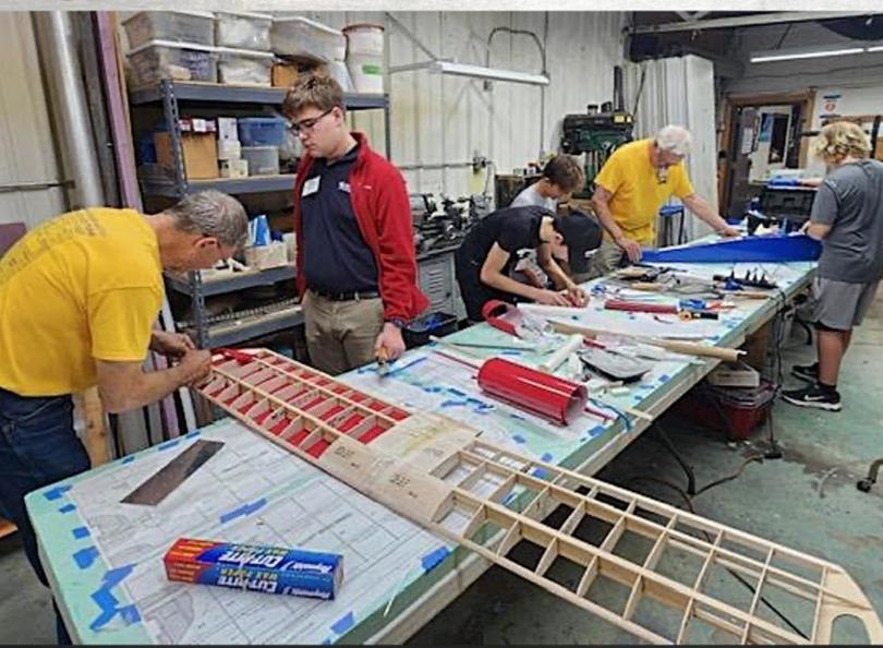
The Build and Fly team is making a lot of progress. The airframe is built and the students are covering it with red, white and blue Monokote.
