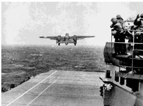
18 April 1942 — USAAF Lieut. Col. James Doolittle led 16 North American Aviation B-25 “Mitchell” bombers on the Tokyo raid. Twenty-four B-25Bs were modified for the mission. Armor was removed; the remote control lower turret was replaced by a 60 gallon fuel tank. A 225 gallon tank in the bomb bay in the bomb bay and a 160 gallon collapsible tank in the crawl way above the bomb bay were added. These tanks increased the fuel capacity from 694 gallons to a total of 1,140.
