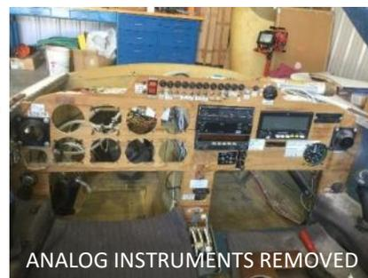
ANALOG INSTRUMENTS REMOVED
