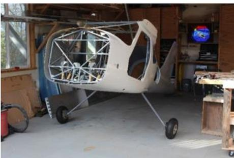
While waiting for the hinge order to arrive, I skipped ahead and started installing the tricycle landing gear. Drilling through 1.5 inch hardened steel is lots of fun. I spent half of the time re-sharpening drill bits. It was exciting to see the fuselage transition to a tail dragger, and then a tricycle geared airplane that rolls around.
