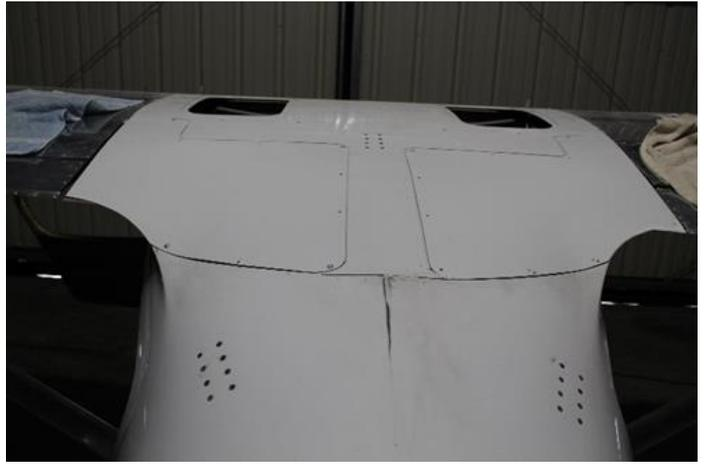
For a change, the elevator tip fairings fit properly and are nearly done. Just waiting on some ordered nut plates to complete the installation.
