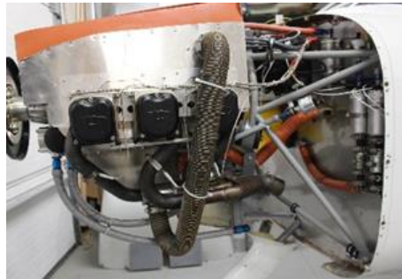
HEAT/DEFROST AIR HOSES
