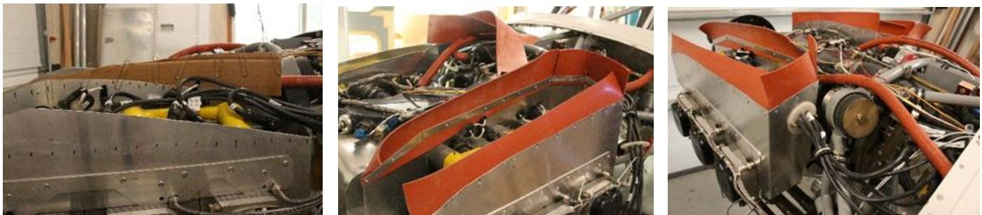
The last project of the month was installing a cabin heater muff on the exhaust pipe and routing a hose to the firewall valve. The muff consists of a shroud around a portion of the exhaust pipe that has a stretched spring wound around it to increase surface area. There is an outside air source hosed to the muff inlet. The air is heated through the muff and exits to the firewall mounted cabin heat/defrost/bypass valve.
