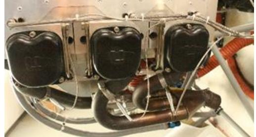
I fabricated the oil cooler hoses and installed them between the engine oil filter and the remote oil cooler.
