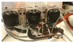
I fabricated the oil cooler hoses and installed them between the engine oil filter and the remote oil cooler.
