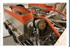
The last project of the month was installing a cabin heater muff on the exhaust pipe and routing a hose to the firewall valve. The muff consists of a shroud around a portion of the exhaust pipe that has a stretched spring wound around it to increase surface area. There is an outside air source hosed to the muff inlet. The air is heated through the muff and exits to the firewall mounted cabin heat/defrost/bypass valve.
