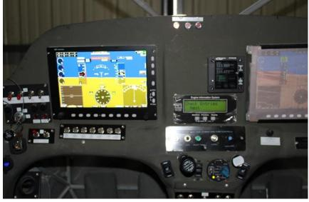
Good news – the com radio/intercom, Bluetooth ADS-B receiver/AHRS system, engine instrument system, auxiliary fuel tank pump timers, and EFIS are mostly debugged and working. Added a resistor to the fuel pressure sensor and rewired a GPS input to the EFIS. The Mode S/ ADS-B TailBeacon X transmitter is not working and will need to be sent in for repairs (bought used, "working when removed").
