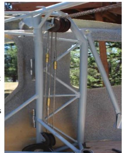
Next and last project for the month was repeating the frustration, by installing the aileron cables and adjusting them to go in **opposite** directions in different amounts (22.5 degrees up and 17.5 degrees down) at the same time. Fortunately the days were long on light, and after lots of adjustments, that job too was done.
