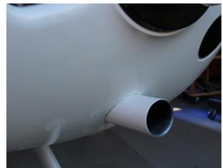
I decided on a 3” circular inlet opening through the lower cowl using a piece of 3” ABS pipe, and glassed it to the lower cowl. It will connect to the oil cooler plenum with a short piece of hose.
