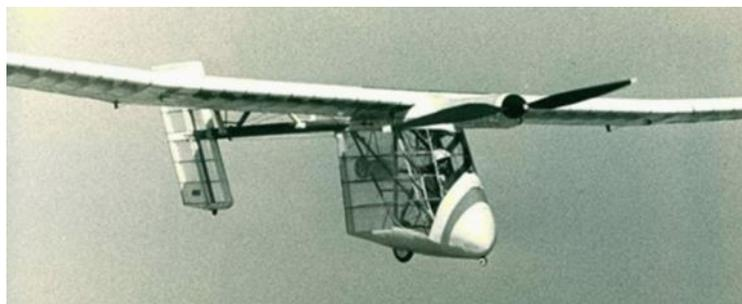
The airplane was designed by Dr. Paul MacCready, Cal Tech, who also designed the Gossamer Albatross, the first human powered plane to cross the Channel. Weighing just 210-pounds, the 47 foot wingspan Solar Challenger is powered by 16,128 photovoltaic cells on the wings and tail that convert solar energy to electricity, which drives the 2.7 horsepower motor. The aircraft does not have any battery back-up power
