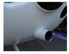
I decided on a 3" circular inlet opening through the lower cowl using a piece of 3" ABS pipe, and glassed it to the lower cowl. It will connect to the oil cooler plenum with a short piece of hose.
