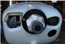
shape, glass, remove foam and glass again. I still have the other side to do, plus closing off the two lower cowl openings.
