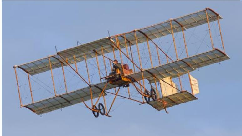
Top photo: A Supermarine Spitfire makes a low pass over the crowd at a Shuttleworth airshow. Above: A replica Bristol Boxkite flies low and slow. Note all the wire bracing.
