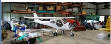
Chris Akin has purchased a partly finished project. The airplane is a Merlin PSA (Personal Sport Aircraft) a single place all metal, high wing, LSA. This one is powered by a two cylinder, four cycle HKS motor. For more information on this diminutive airplane visit the Merlin website. This little airplane looks like it would be a lot of fun and the operating expenses would certainly be easy on the budget.
