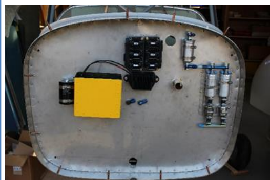
Battery box, 13 pieces, 50 rivets
