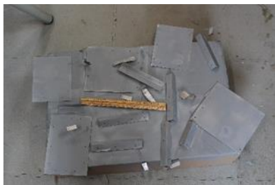
Battery box, 13 pieces, 50 rivets
