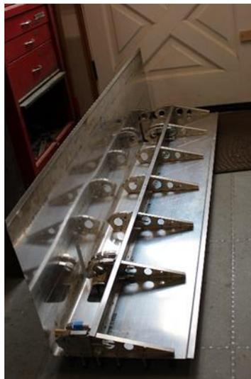
A partly assembled aileron.
