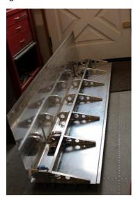
A partly assembled aileron.
