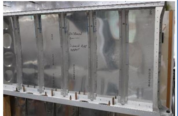
There also a couple of one-inch aluminum strips that reinforce the upper main spar near the strut attach fitting, another 130
