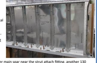
There also a couple of one-inch aluminum strips that reinforce the upper main spar near the strut attach fitting, another 130
