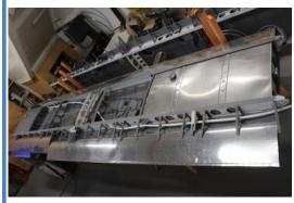
The last step to complete the wing components is installing the five standard, plus one extra inspection hole covers. This is what I am working on now.
