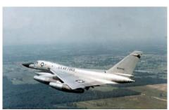
Electric J79 engines in underwing pods powered the supersonic bomber. It carried a single nuclear weapon plus fuel in a combination bomb/fuel pod underneath the fuselage instead of the usual bomb bay. Four external hard points were added later, enabling it to carry up to five weapons.
