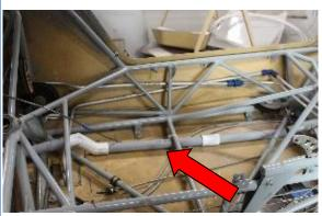
I installed a PVC conduit under the seats to the aircraft front for all the wires to the aft fuselage. These include the magnetometer, electric elevator trim and position sensor wires, and wires for the uAvionix tailBeacon X.
