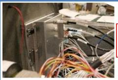
I started hooking up the EFIS by connecting the static and pitot lines. This was made much easier than for previous planes by using quick connect fittings instead of slipon hose fittings and clamps.
