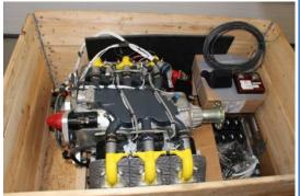
at 200 hp at 3300 rpm for 5 minutes and 185 hp at 2900 rpm for cruise. It is designed to use 93 octane mogas with ethanol or 100 LL and weighs about 30 pounds less than an O-320. I have also purchased a matching 3 blade Airmaster electric controlled constant speed propeller yet to be delivered.
