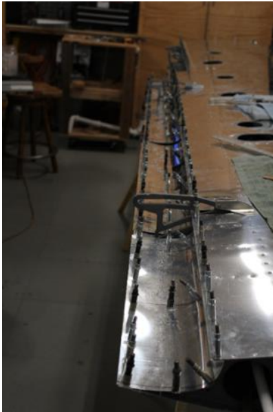
Right Wing Cove ready for rivets
