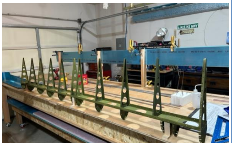
Work on the right flap assembly has been paused while I wait for warmer weather. I need to corrosion proof the nose skins.
