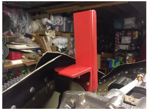
Prop Balance Instrumentation Mount I made for my engine on the RV7 - TAW
