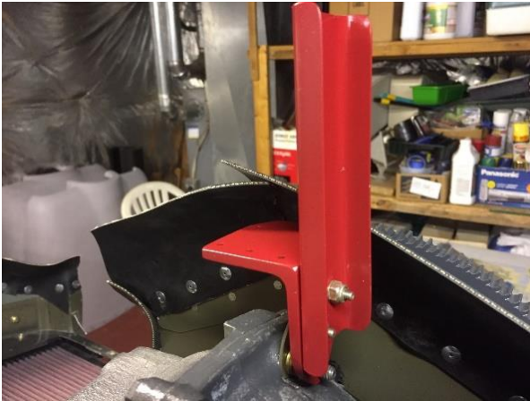
Prop Balance Instrumentation Mount I made for my engine on the RV7 - TAW
