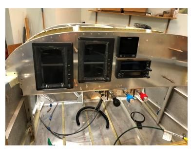
The second picture shows the panel without the avionics but with most switches and holes. Over to the right will be a small glovebox and below that a dropdown fuse panel. I am trying to keep the panel as removable as possible since I do plan to have it professionally painted and labelled.
