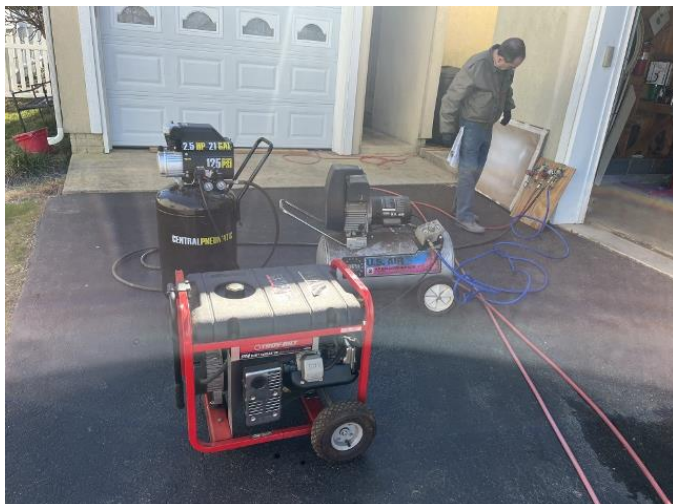
Dual compressors powered by a ten-hp generator.
