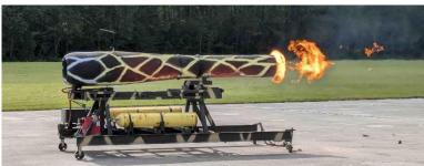
Th\_e flying began at noon and ended at 3:45. Just about everything flew except the Airacobra which aborted takeoff for a mechanical issue. During a break in the flying, they demonstrated a V-1 buzz bomb pulse-jet motor, running it on a stand at low power for over a minute until it glowed red.
