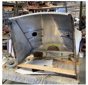
The upper cowling appears to fit properly. On the other hand, the lower cowling doesn't fit at all. Photo 3 shows the inside of the lower cowling. Wooden bracing have been temporarily clamped in place to keep the cowling sides located where they need to be to fit around the new engine. The lower center section of the cowling needed extensive metal work. This can also be seen in Photo 4.
