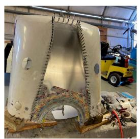
Photo 5 shows the finished lip. The aluminum lower cowling center section has been riveted and external doubters for the cowling attach support have also been riveted. At this point, we are awaiting new support isolators for the cowling. This existing cowling had cracks in the aluminum skin where the cowling attached to the brackets so this is fixed.
