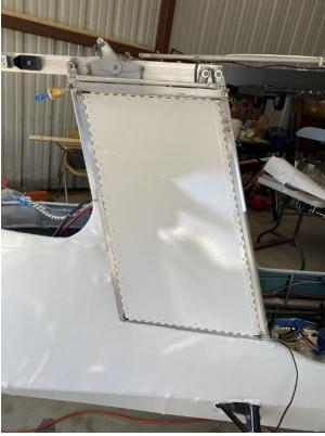
Installing the Engine Accessory Compartment Panels: Held in place by piano hinges on four sides. Fabric, glue and paint thickness buildup are causing interference in fit dimensions. The retaining hinge pin cannot be fully inserted on the right side cover. The Left Side Cover does not have this issue. Working on resolving the fit issue.
