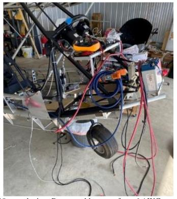
19-strand wire. Battery cables went from 6 AWG to more robust 4 AWG obtained from Battery Cables USA. The 15-amp battery charging circuit 18 AWG wiring was replaced with 14 AWG wire. Extension cable for the EGT and CHT sensors went from 22 AWG to 18 AWG per the factory call-out.
