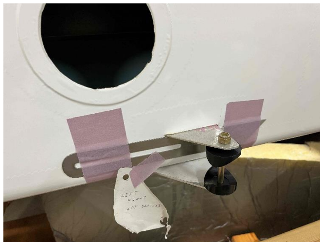
Lift Strut Attachment Brackets - Temporary Mount
