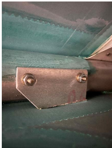
Lift Strut Attachment Brackets - Temporary Mount
