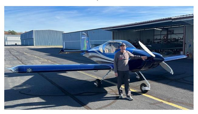
I first flew my RV-14A, N9314A, on November 24 and completed "*initial*" Phase 1 test on February 10. I specify "initial" because I will need to re-enter Phase 1 to test the aircraft's aerobatic capabilities after I get some current aerobatic training.
