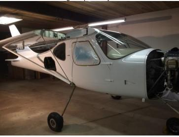
Fuselage, painted. Front windshield installed by Airlink.
