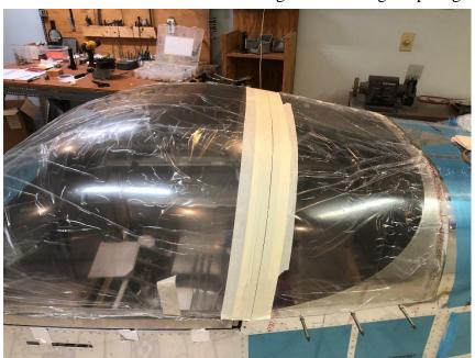
prevent cracking while it is being cut (with cutting wheel in die grinder)--so I had to increase my carbon footprint to heat the shop to about 80 deg. Cut edges are smoothed immediately after cutting to eliminate stress risers.
