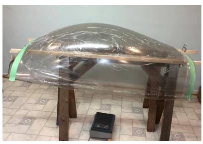
This roll bar establishes the point where the canopy splits into the tip up portion and the fixed "rear window". The picture shows the bubble marked off for making this "big cut" as shown by the thin gap between the two rows of making tape.
