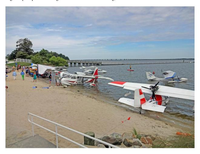
There are two kinds of seaplanes, one with floats and flying boats. A flying boat has a fuselage shaped like the hull of a boat. My training was in a Progressive Aerodyne Searey, a flying boat. The Searey is a two-seat Light Sport Aircraft (LSA) that has a high wing, a Rotax engine with a pusher propeller and side-by-side seating. The conventional landing gear retracts up near the wing struts and
