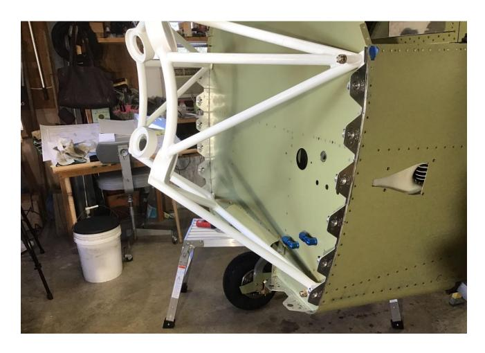
I'm now working on tail light/strobe, static air and mounting ADHARS in fuselage. Should be able to cut instrument panel, install avionics and mount engine next month. It seems like I'm getting close, but probably have 95% to go as the old saying goes
