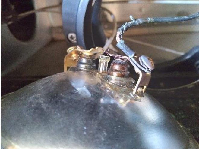
Ground wire to the taxi light was bare, a little corroded, and brittle. The screw was also a little loose resulting in intermittent operation.
