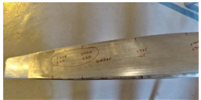
Prop was stripped and measured, revealing excessive wear on both ends about 6-8 inches inboard from the tips.
