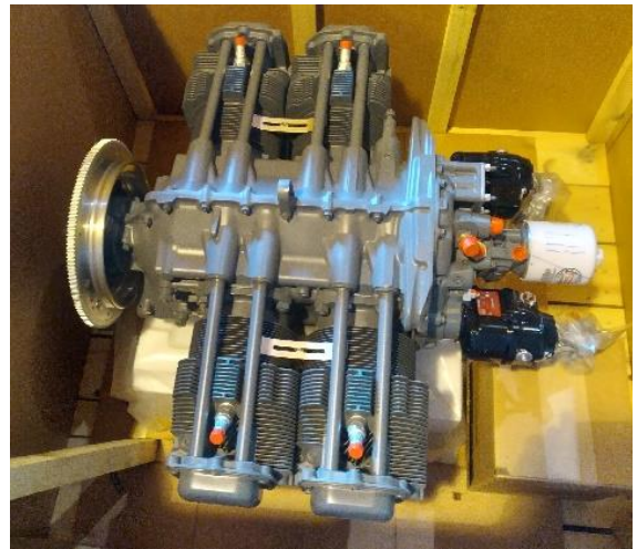
Shiny zero-time engine still in the crate waiting for installation.
