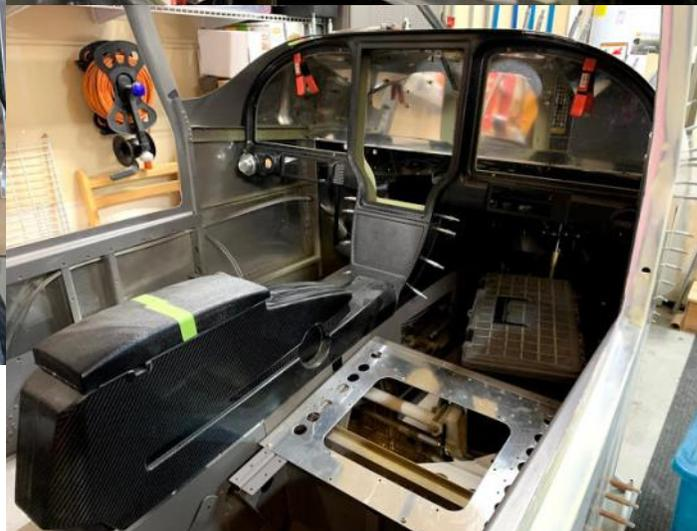
the tasks I took picture of below I also managed to finish riveting the top skin on the inside. I forgot to do this when Travis was here so finished up the last 8 rivets. I also epoxied in the two forward Naca ducts.
