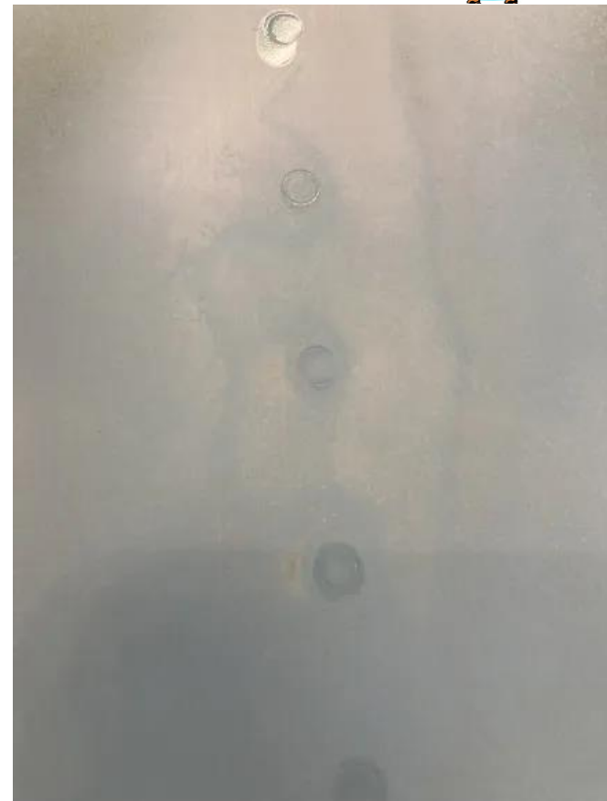
Detail of the final blue primer over gray primer over zinc chromate... with one of the high spots that sanded through for good measure.
