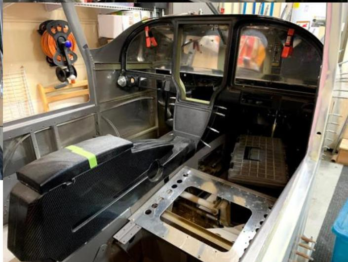
the tasks I took picture of below I also managed to finish riveting the top skin on the inside. I forgot to do this when Travis was here so finished up the last 8 rivets. I also epoxied in the two forward Naca ducts.
