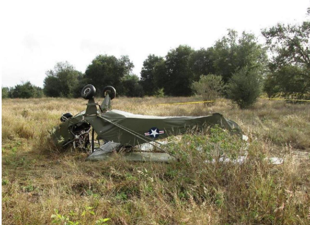
**Kitfox- Idaho:** During the landing roll, the left main landing gear slowly collapsed forward. During a Postaccident examination of the airframe it was revealed that the left main landing forward gear tube had collapsed, which resulted in substantial damage to the landing gear mounting bracket. (2/7/2017)
