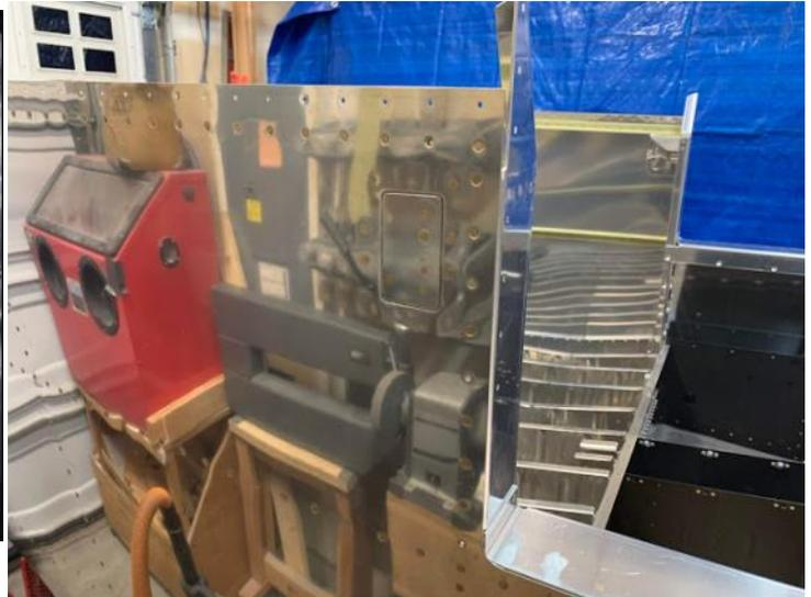
The only steps left for this section is to rivet in two side ribs (which should go pretty quickly) and to install the main landing gear weldments. That last step will probably be a bummer since it involves many bolts and holes that all have to line up properly...and never do...depending on the temperature in the garage, the phase of the moon and how I position my head while banging it on the wall. :-)
