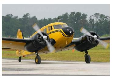
Powerplant: 2 × Jacobs R-755-9 seven-cylinder, air-cooled, radial piston engine, 245 hp (183 kW) each
