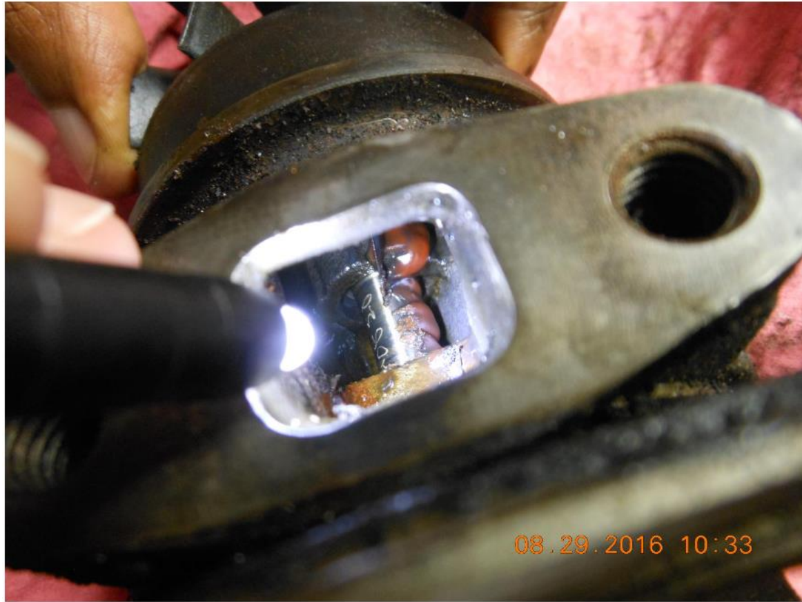
Photo 5 – View of foreign material in center turbo housing
