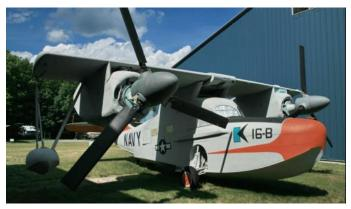
**General characteristics** Crew: 2 Length: 38 ft 4 in (11.68 m) Wingspan: 34 ft 0 in (10.36 m) Height: 19 ft 2 in (5.84 m) Empty weight: 6,500 lb (2,948 kg) Gross weight: 8,000 lb (3,628.74 kg) Powerplant: 2 × General Electric YT58-GE-2A turboshafts, 1324.9 hp (988 kW) each Propellers: 3-bladed Kaman, 14 ft 10 in (4.5 m) diameter
