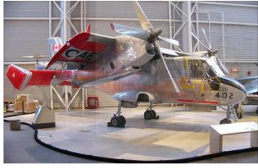
**General characteristics** Crew: 2 Capacity: 12 passengers Length: 47 ft 3.5 in (14.415 m) Wingspan: 34 ft 4 in (10.46 m) Height: 14 ft 3 in (4.34 m) Wing area: 233.3 sq ft (21.67 m2) Airfoil: NACA 633-418 Empty weight: 8,417 lb (3,818 kg) Max takeoff weight: 14,500 lb (6,577 kg) (STOL), 12,600 lb (5,710 kg) (VTOL)
