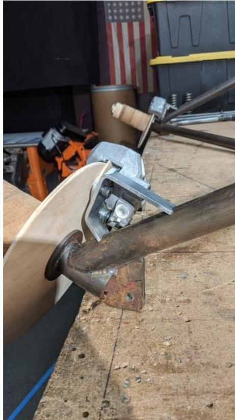
clamp the elevator horns together while drilling. This worked out wonderfully! You can see the 3D printed block with the bolt installed after drilling.
