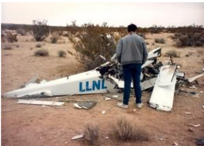
D-1 wreckage after crashing on its 19 th flight due to servo failure
