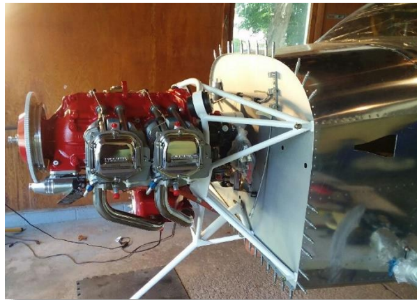
Lycoming O-360 mounted on the RV
